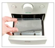
2. Place sealing film on plate.
