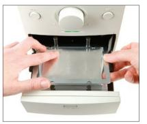
3. Place seal frame on sealing film.
